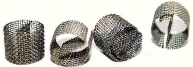
Figure 1- A photograph of 1/8" Dixon rings as tested within this work.
